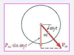
• Evaluate the magnitude of the periodic force due to the motor unbalance. Determine the vibration amplitude from the frequency ratio at 1200 rpm.
