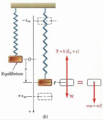
If a particle is displaced through a distance  $x_m$  from its equilibrium position and released with no velocity, the particle will undergo *simple harmonic motion*,
