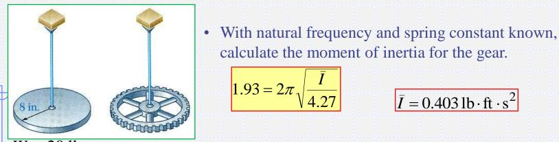
calculate the moment of inertia for the gear.
