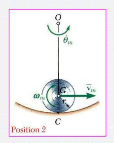
$$T_{2} = \frac{1}{2}m\overline{v}_{m}^{2} + \frac{1}{2}\overline{I}\omega_{m}^{2}$$
