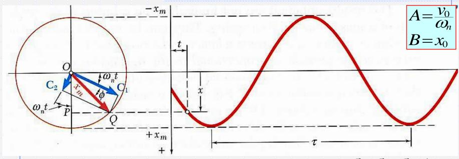
• Displacement is equivalent to the x component of the sum of two vectors  $\vec{C}_1 + \vec{C}_2 = \vec{A} + \vec{B}$  which rotate with constant angular velocity  $\omega_n$ .
